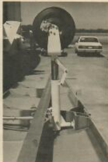
The retractable gear assembly is simple, reliable and easy to maintain.
