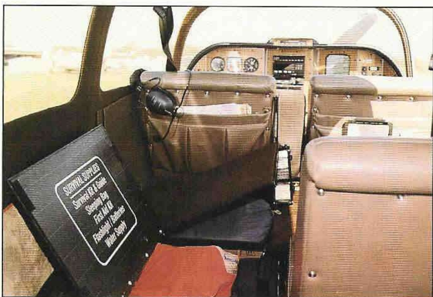
N360EZ's cabin had a flat floor covering two storage bays and could be used as a 74" long bed. A 4th seat could be installed as an alternative.
