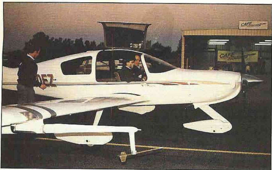
CAFE Barograph, pitot-static and boom mounted on right wing for first data flight at dawn on 9/20/97. Note large, gull-wing cabin door and rear baggage door.
