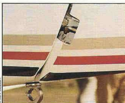
A rudder stop bolt was set to limit travel to 20° on each side.
